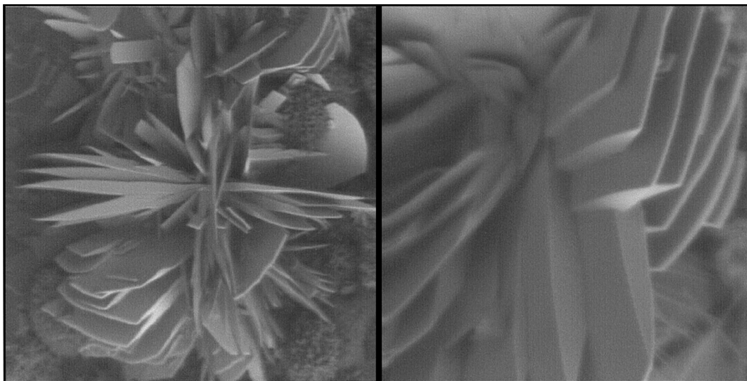
Fig. 1. Backscatter scanning electron micrograph of KNAURSI found on the surface of 51S waste glass subjected to vapor hydration for 60 days at 200°C and 100% RH. Field of view = 328 \mu\text{m} .
